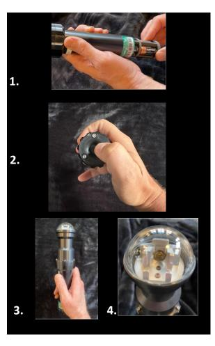
**STEP 1.** Remove threaded end cap from device and insert 123 battery carriage. Replace end cap securely.
